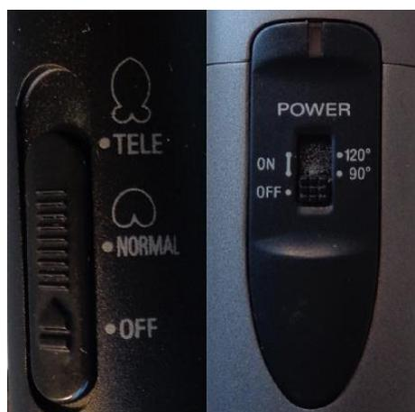
Figure 3.8. Microphone switches to alter the microphone's directionality
